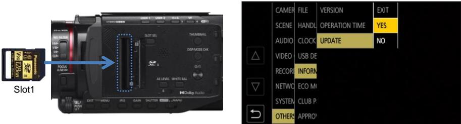
5. The operation indicator lamp will flash, and after about 30 seconds, the unit will automatically restart. When the message "Update successful" appears, press OK..
