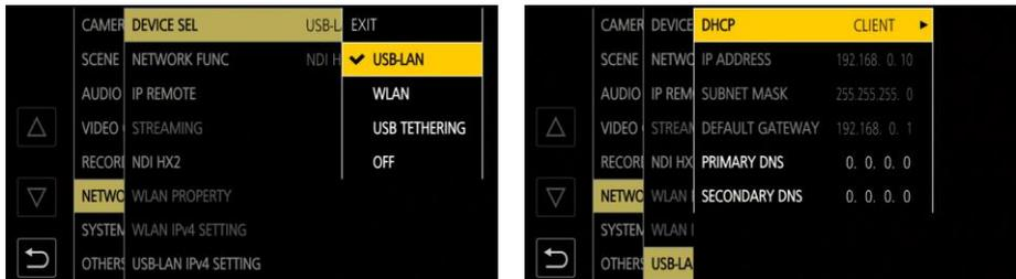
Example of the setting screen when connecting to USB-LAN
