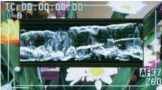
Built-in waveform monitor (WFM)
