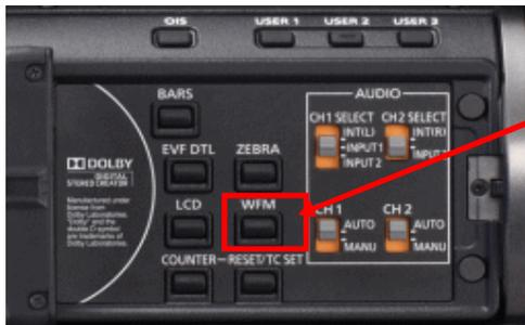
Turn ON / OFF WFM / VSC display with the "WFM" button.
