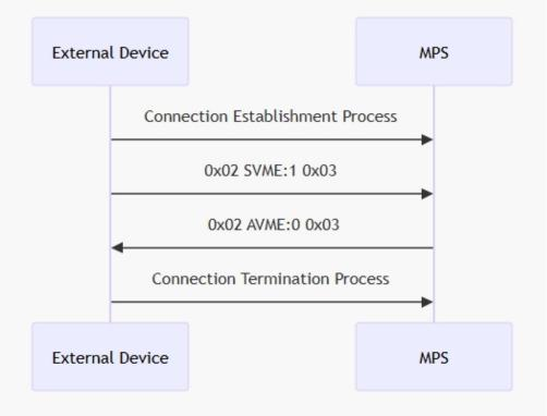
In a TCP connection, an external device sends a control command, and the MPS sends a response command (including an error response). If the external device no longer needs to send the command after receiving the response command, terminate the connection for TCP communication.
