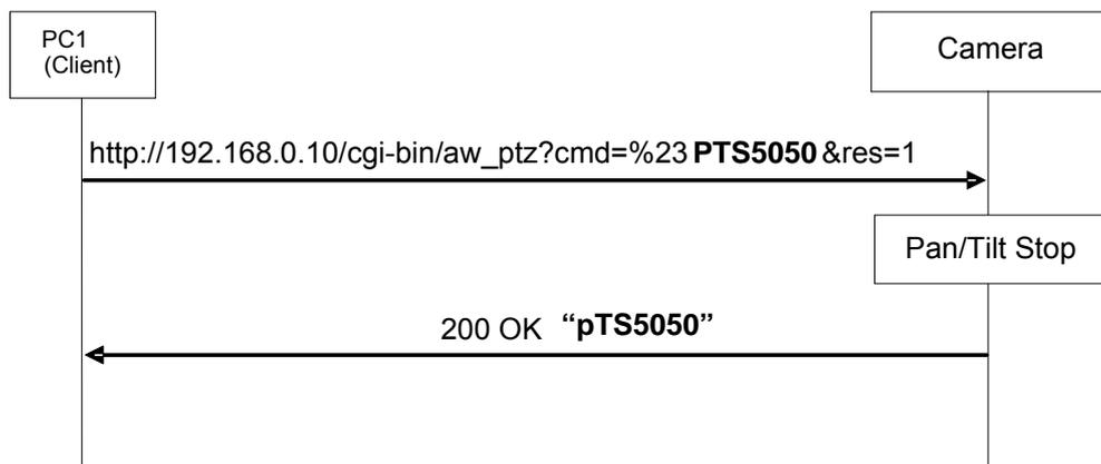
Fig.3.1-1 Command sequence of System control
