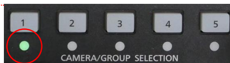
(Status Indicator Lamp ... Shows the camera's power status)
