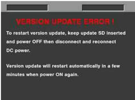
If the power supply is shut down on the way to update or above error operation happens, turn the power OFF/ON then restart the write function start again in a few minutes.
