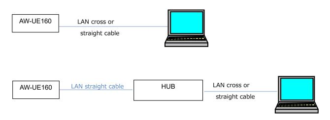
Select an IP address for the personal computer within the private address range while ensuring that it is different from the address of the unit. Set the subnet mask to the same address as the unit.
