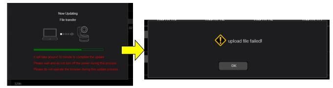
If you disconnect the LAN cable or the power supply from the following screen please connect the LAN cable or the power supply again.
