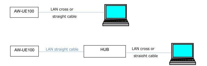
Select an IP address for the personal computer within the private address range while ensuring that it is different from the address of the unit. Set the subnet mask to the same address as the unit.
