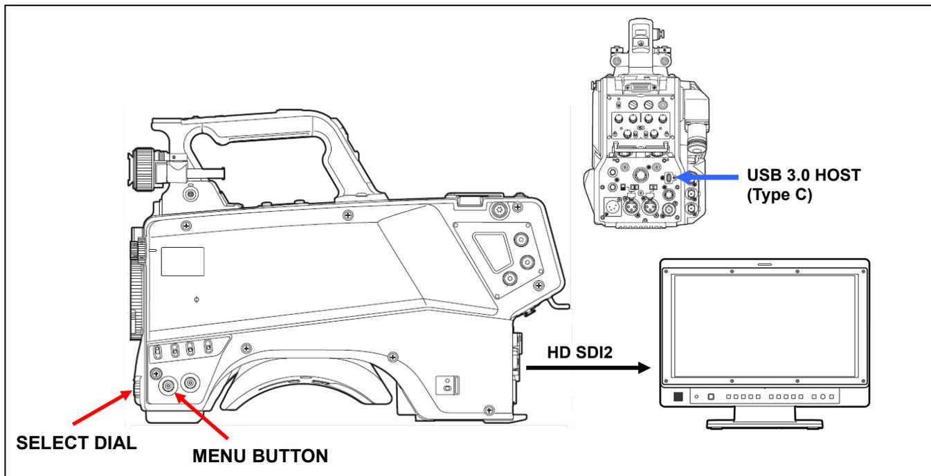
3. Select "MAINTENANCE" in "ALL MENU 2/2" and press the SELECT DIAL button to open the MAINTENANCE menu screen.
