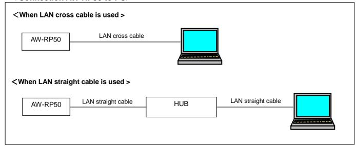
The LAN cross cable is used when connecting a personal computer directly to the unit's LAN connector for IP control, and the LAN straight cable is used when making the connection through a switching hub.
