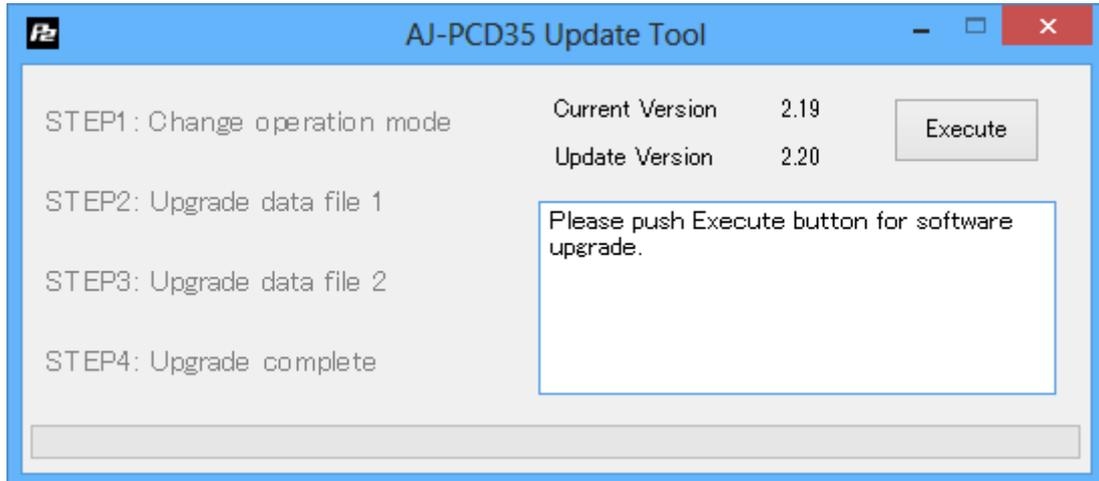
If the screen is displayed as follows, AJ-PCD35 is not recognized. Please check the connection with PC again.
