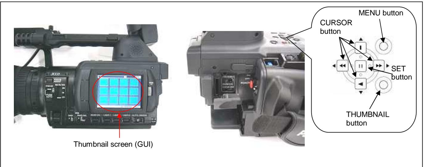
3. Press the **MENU** button to display the menu. Use the **CURSOR** buttons to select the item “**OPERATION**” and press **SET** button to open the OPERATION menu.
