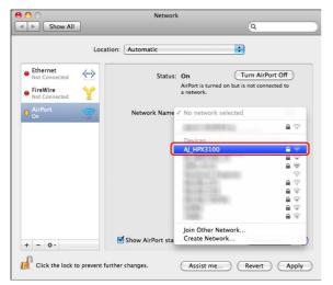
6 Enter the WPA2 encryption key (factory default: 01234567890123456789abcdef) set in the P2 cam in response to the password request, enter a check for [Remember this network] and click OK
