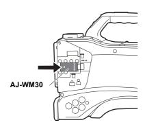
3 Replace the cover removed in 1, and fasten the 2 screws.
