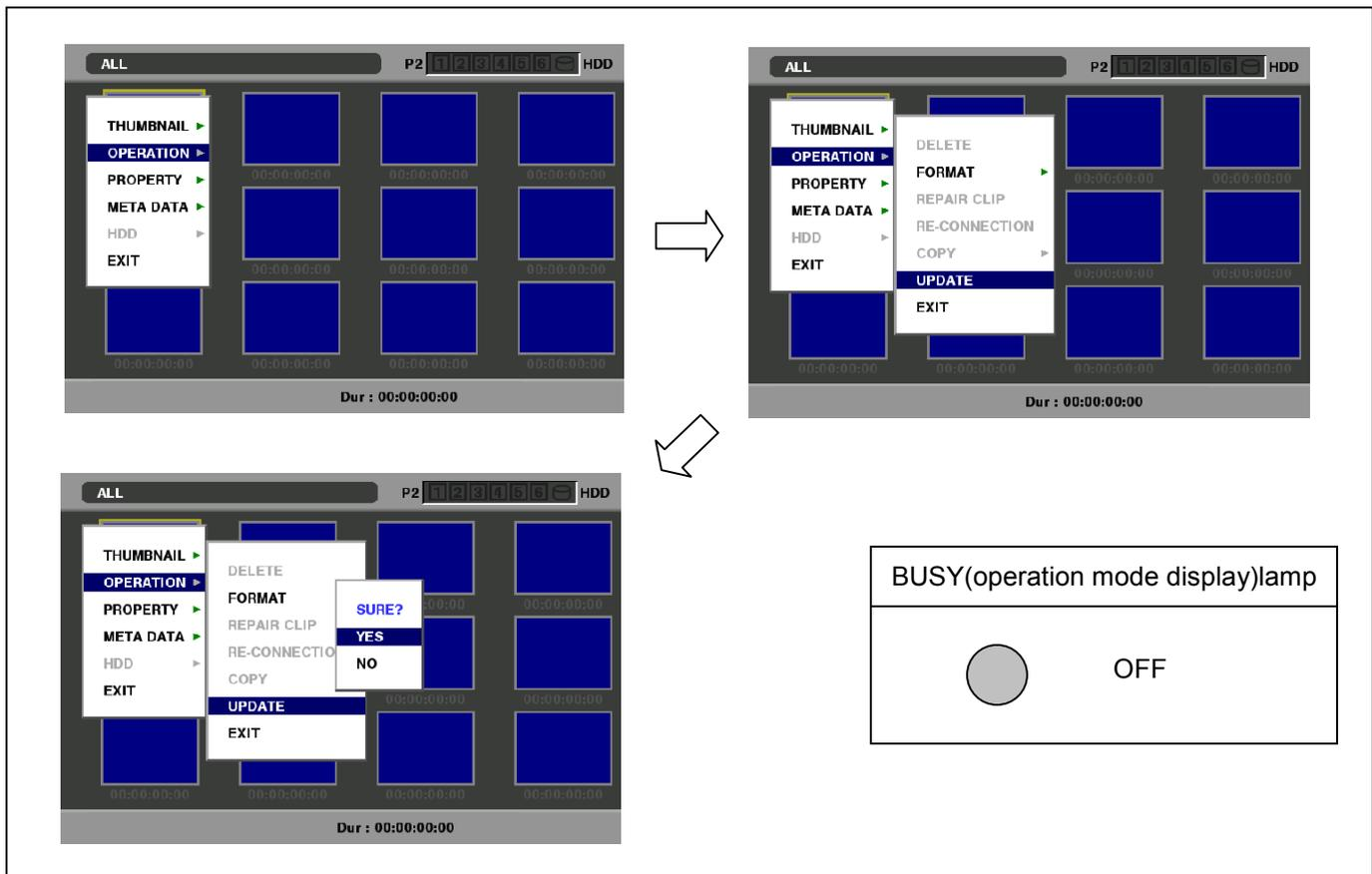
4. Update program is started and the message “**PREPARING FOR UPDATE**” appears on screen. In this timing, it is doing preparation such as the confirmation of the data of the updating. In this time, BUSY(operation mode display)lamp is turned off.
