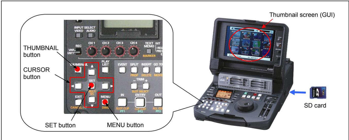
2. Press the **MENU** button to display the menu. Use the **CURSOR** buttons to select the item “**OPERATION**” and press **SET** button to open the OPERATION menu.
