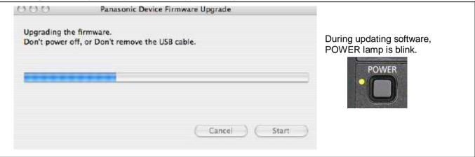
**3-9.** The following window is displayed when the software update is completed. Click the "OK" button and turn off the power of AG-HMR10 /AG-MDR15. Disconnect the USB cable.
