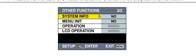
5. Press the PLAY/STILL or STOP button to select the "YES". And press the ENTER button to display the version number on the SYSTEM INFO screen.
