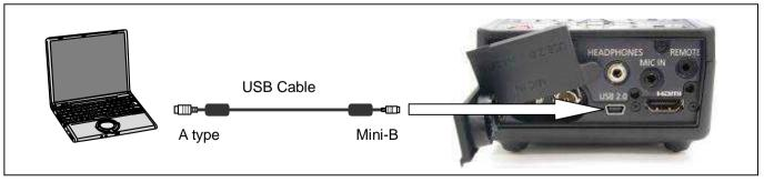
**3-7.** The following window is displayed after the USB connector of AG-HMR10 /AG-MDR15 is connected to MAC with USB cable. Clicking "Start" button, software update is started.
