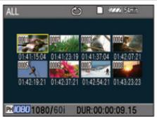
Used for the playback of clips that are recorded on the SD Memory Card. Also, clip management operations, such as deletion and protection, can be performed on the thumbnail display screen.
