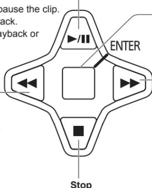
Press during playback to stop playback and return to the thumbnail display screen.
