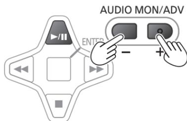
The images are advanced when the + button is pressed, and reversed when the - button is pressed, in about half-second intervals.
