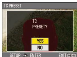
With this portable recorder, the time code value is adjusted in accordance with the recording format and frame rate. When shooting is performed with the recording format set to 1080/24P or 720/24P, recording is performed 4 frames at a time. For this reason, if you change the recording format or frame rate, it may result in discontinuity from the last time code value of the previous recording. (Only when [SYSTEM FREQ] is set to [59.9Hz])
