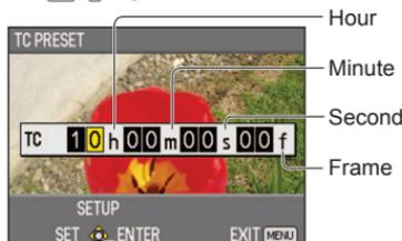
Example: To set 10 hours, 23 minutes, 46 seconds, frame 20, select the time code value "10h23m46s20f."
