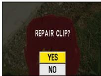
Select [YES] to begin repairing. When repairing is complete, "REPAIR FINISHED" will be displayed, and the display will switch to the recording paused screen.
