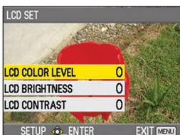
LCD COLOR LEVEL: Adjusts the color density of the screen.
