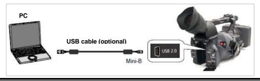
①-2 The following window is displayed after the camera recorder is connected to PC with USB cable. Click the [Start] button and the software update is stated.
