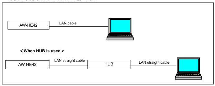
The LAN straight cable is used when making the connection through a switching hub.
