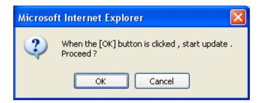
9. When you click the OK button on the confirmation screen, the message "Sending firmware file..." is displayed. The firmware file is transferred from the PC to the camera.
