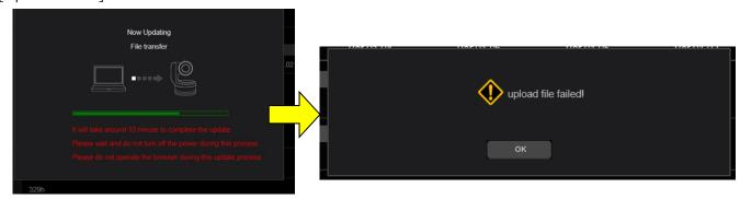
If you disconnect the LAN cable or the power supply from the following screen please connect the LAN cable or the power supply again.
