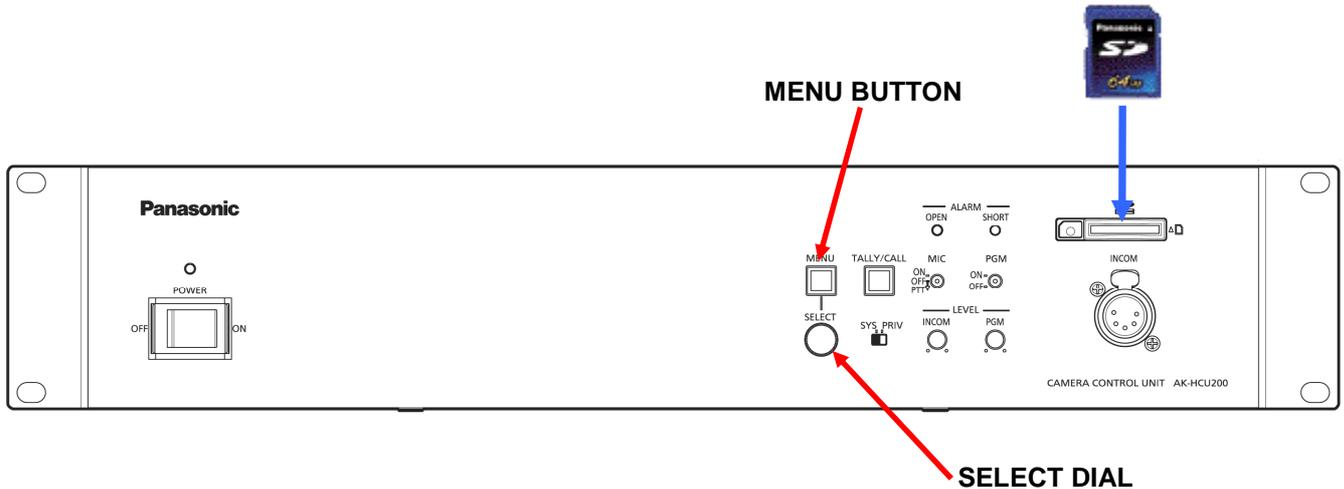
4. Select “**MAINTENANCE**” and press the **SELECT dial** button to open the MAINTENANC menu screen.
