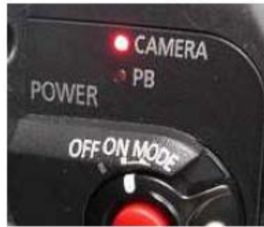
Mode indicator lights when update is finished.
