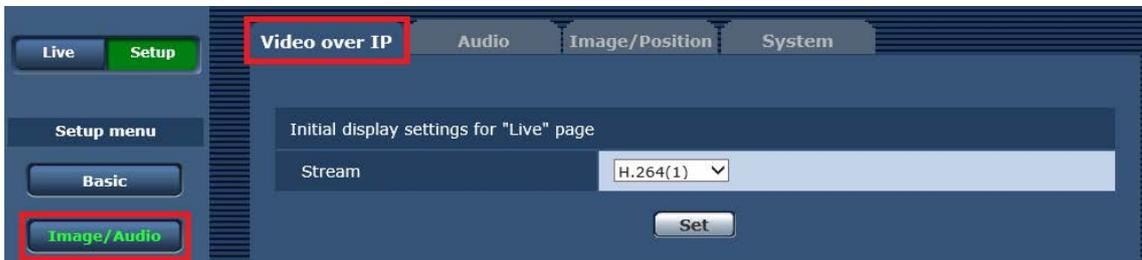
8. Set the operation of H.264 (1) through H.264 (4) in the [Video over IP] tab. When using this software, it is necessary to make settings so that the following parameters satisfy the conditions described here. After setting the parameters, click the Set button and save the settings.
