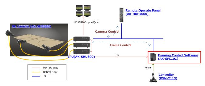
AK-SHB800 is an 8K multipurpose camera. Also, it is an IPU (Imaging Processing Unit) that performs video signal processing. 8K videos shot with AK-SHB800 can be transmitted to AK-SHU800, wherein video signal processing can be done, by connecting both the devices through Optical Fiber.
