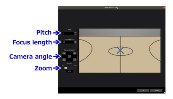
Opening the setting screen when a remote camera is connected will display the captured video. There is an x mark in the middle of the picture to make it easy to ascertain where the center is. Pitch and focus length can be set using the corresponding settings for the 8K camera when the captured frames are taken from a remote camera through an 8K camera. Additionally, the camera angle can be similarly specified within the shooting position of the 8K's angle of view.
