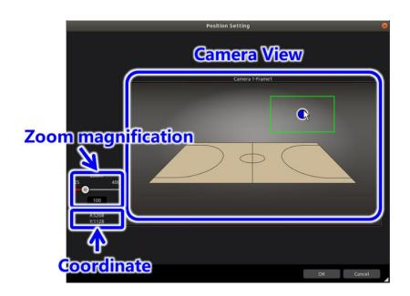
In the fixed position setting screen, position of captured frame can be set by clicking on the Camera View screen. At this time, central position of captured frame is displayed in coordinates column as 8K angle of view (7680x4320).
