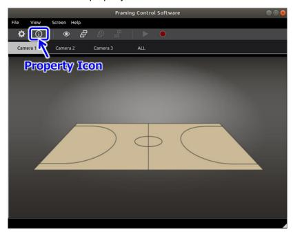
In the property screen, item for reference is displayed to the left side as shown below. There is Network as the item for reference. Further, menu bar and the tool bar are disabled when property screen is displayed.
