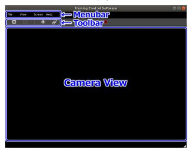
In the Menu bar, various menu operations can be carried out. Refer to **Menu Configuration** for details. Menu operations are possible only from the view screen, the preset screen screen. From the Toolbar, you can view the **Settings Screen** and **Property Screen**, and transit to the **Preset / Tracing Memory Screen** and **Tracing Memory screen**. Other buttons are not currently useable, but are scheduled to have functionality added. For more details, refer to each item.
