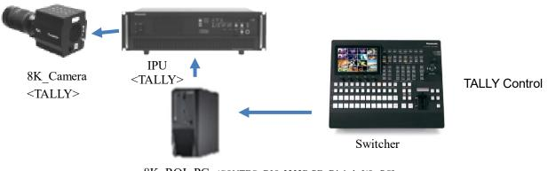
8K\_ROI PC (CONTEC DIO-3232B-PE Digital I/O PCI Express card 32ch/32ch inserted)
