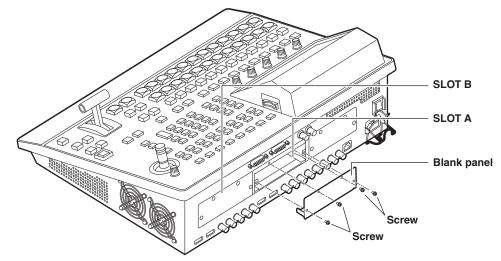
③ Insert slowly, following the guide rails in the slot on the main unit.
