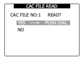
NOTE: The CAC file that can be installed in the Camera is up to 8 files. If 8 files are loaded, "READ NG CAC FILE FULL" appears. Delete any existing files before installing a new file.
