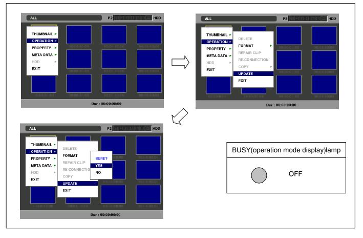
4. Update program is started and the message "**PREPARING FOR UPDATE**" appears on screen. In this timing, it is doing preparation such as the confirmation of the data of the updating. In this time, BUSY(operation mode display)lamp is turned off.
