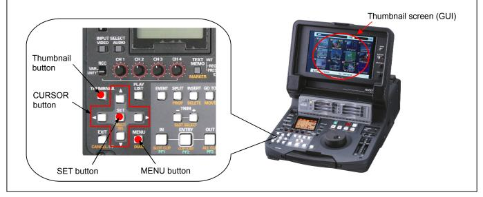
2. Press the **MENU button** to display the menu. Use the **CURSOR buttons** to select the "**PROPERTY**" and press **SET button** to open the PROPERTY menu.
