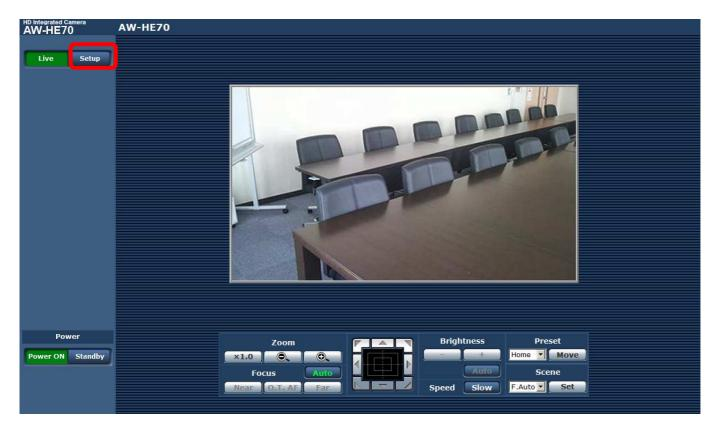
4. Clicking **Setup** button, the following screen is displayed. Click **OK** button on the screen, setup menu is displayed.
